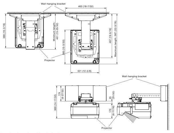
The illustration shows the wall-hanging bracket attached to the projector.
