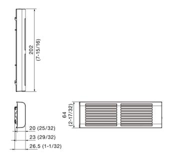
Illustration shows the filter unit attached to the PT-LB2/LB1.
