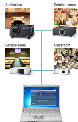
Basic concept of the Multi Projector Monitoring and Control Software.
