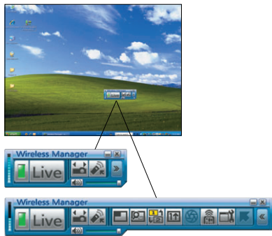
Wireless Manager Control Panel (Launcher) To begin wireless projection, simply use the control panel (launcher) displayed in the PC window.
