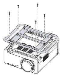
(5) Secure the four adjustable feet that were removed in step (2) to the carrying handle.
