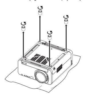
① Place the projector upside-down onto a piece of soft material.
