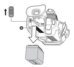
Move the battery release lever in the direction indicated by the arrow and remove the battery when unlocked.
