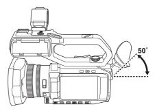
3 Adjust the characters on the viewfinder screen so that they are clearly visible using the diopter adjustment dial **a**.
