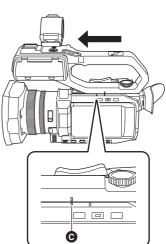
5 While pressing the handle unit mounting screw down, turn it in the direction indicated by arrow 2 until it stops.
