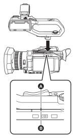
**4** Slide the handle unit in the direction indicated by the arrow.
