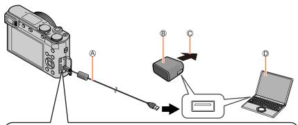
When charging the camera, connect the USB connection cable (supplied) to the [USB/CHARGE] socket.
