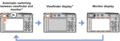
\* When [Eye Sensor AF] in the [Custom] ([Focus / Release Shutter]) menu is set to [ON], the camera adjusts the focus automatically as the eye sensor is activated. Even when [Eye Sensor AF] is set and the camera automatically adjusts the focus, a beep will not sound.
