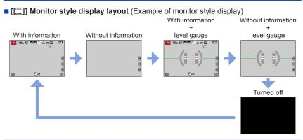
• With [Fn Button Set] in the [Custom] ([Operation]) menu, you can assign [LVF/Monitor Disp. Style] to a function button. Each time you press the assigned function button, the display style of the monitor or viewfinder ([\_\_\_\_]/[\_\_\_]), whichever is currently in use, will change.
