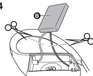
The following instructions are not intended for repairing purposes but for the disposal of this unit. This unit is not restorable once disassembled. When disposing of this unit, take out the battery installed in this unit and recycle it.
