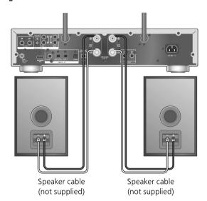
1 Turn the knobs to loosen them, and insert the core wires into the holes.
