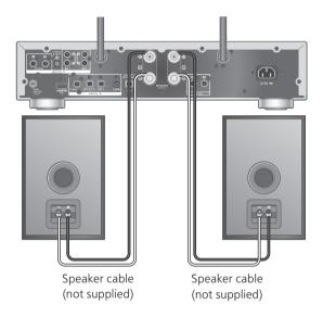
1 Turn the knobs to loosen them, and insert the core wires into the holes.
