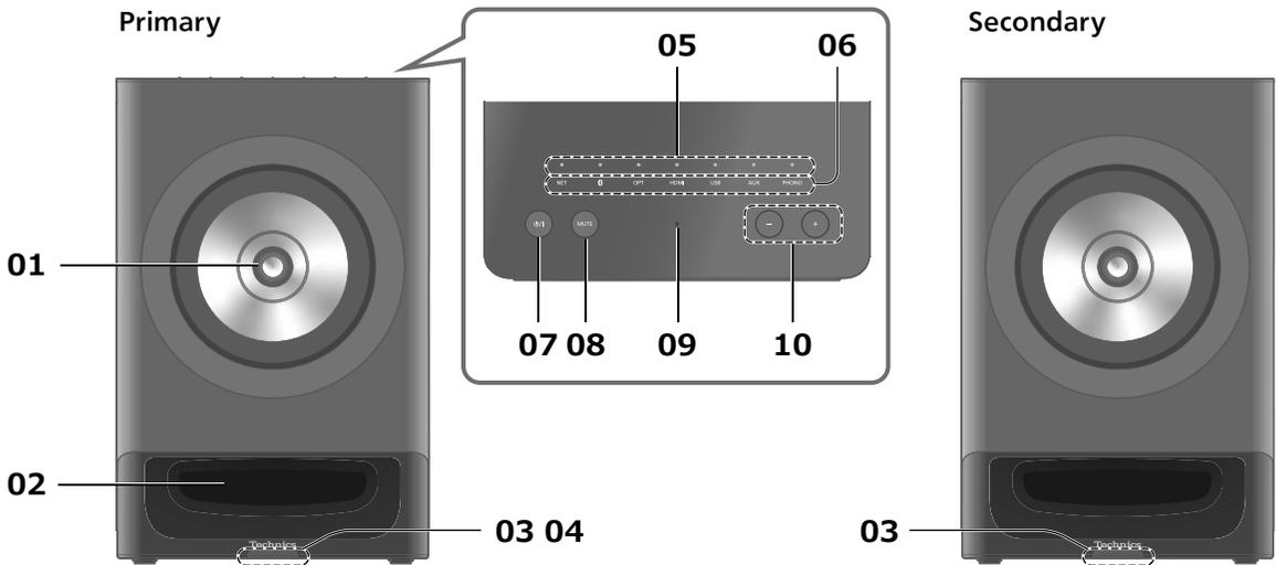
**01 Speaker unit (Coaxial 2-way unit)****02 Bass reflex port****03 Power indicator**
