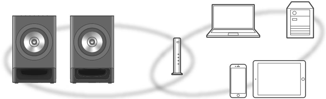
This unit can be connected to a router using a LAN cable or built-in Wi-Fi®. For a stable connection to the network, a wired LAN connection is recommended.
