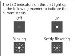
• If an abnormality occurs, all the LED indicators on the top of this unit blink 3 times quickly and then repeat. Press [0]on this unit to turn it on/off. If the problem persists, disconnect the AC mains lead, wait for at least 3 minutes, and then reconnect
